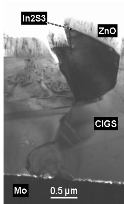
Figure 2: BF-TEM image of a CIGS based solar cell with In<sub>2</sub>S<sub>3</sub> buffer layer (grown at Stuttgart University) shows uniform coverage of the CIGS layer.
