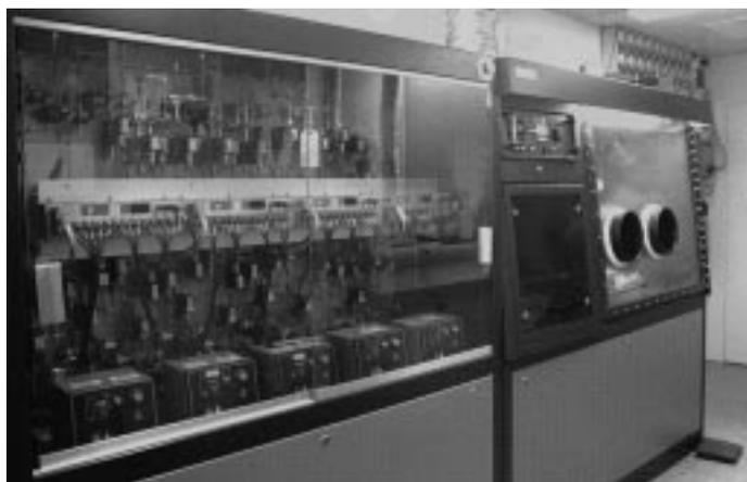
Photograph of our LP-MOVPE system with gas mixing cabinet, reactor and glovebox for loading (from left).
