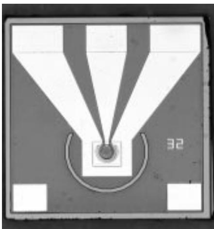
Photograph of photodiode chip with  $\varnothing$  32 $\mu\text{m}$  diode and electrical coplanar transmission lines for high speed applications
